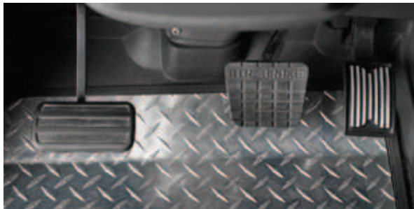
COMFORTABLE PEDALS: The pedals on the Mack® Granite are suspended above the cab floor with the accelerator and brake pedals mounted in-line to reduce operator effort while driving. The clutch pedal is available with air assist, lowering the pedal and greatly reducing driver effort. When combined with our new deep cab and strategically placed seat and steering column, drivers conserve energy and work more productively.
