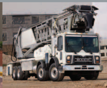
CONCRETE CONVEYOR BELT
