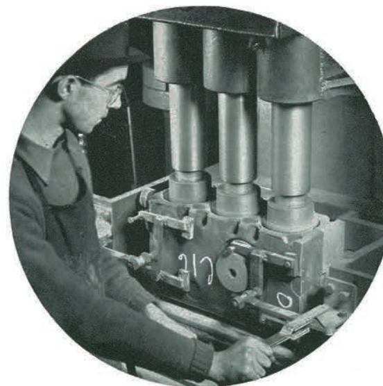
Uniform thickness and perfect alignment of cylinder walls is assured by precision boring every core used in cylinder block casting.
