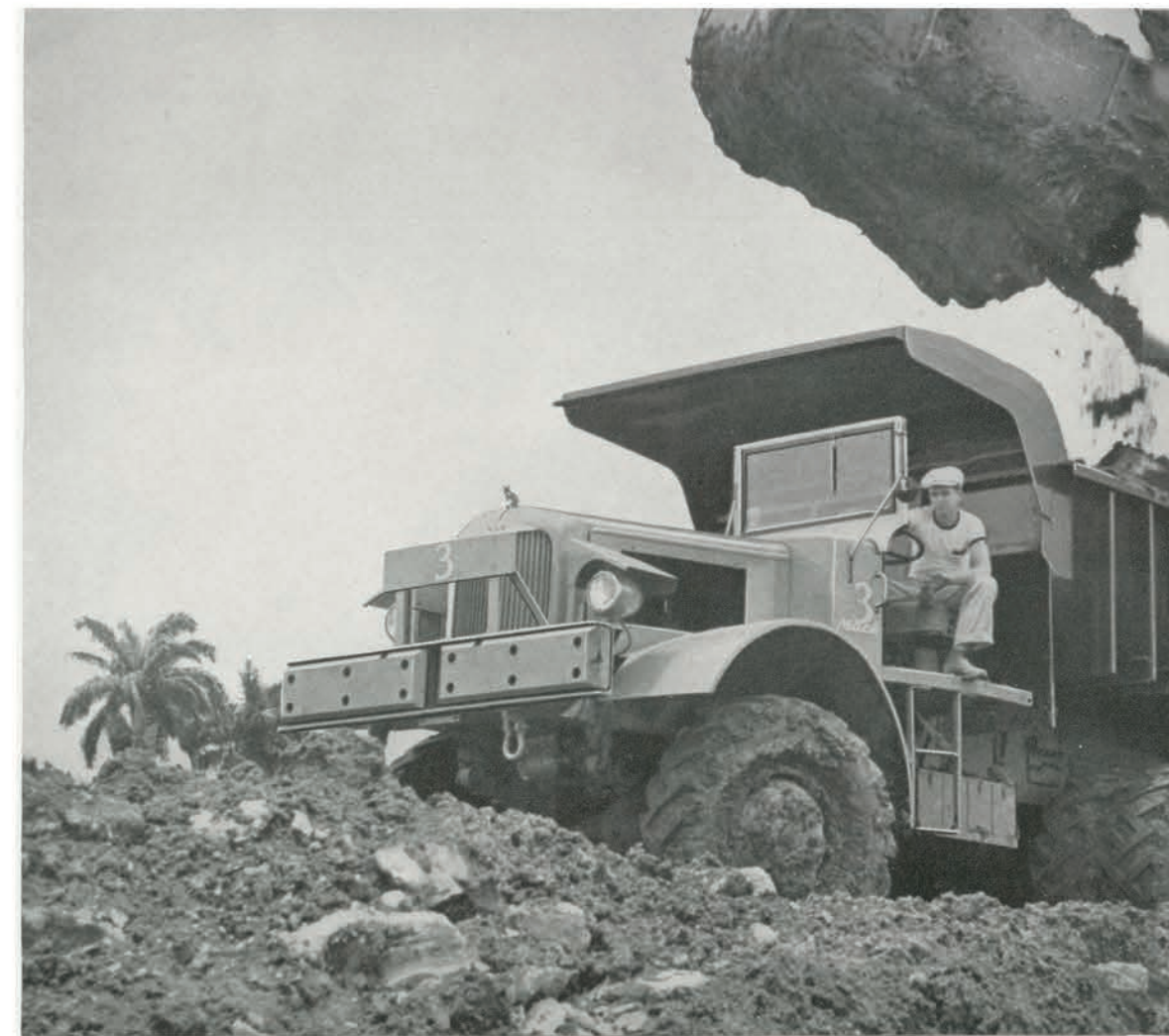
Monster Mack swamp dumpers, now working for Wunderlich-Okes Construction Co. on Panama Canal Third Locks Project, tip the beam at 30 tons when loaded. They're close to 12 feet wide and are powered by 150 h.p. diesel engines. Designed for operation in yielding swamp and muck these big fellows have drive on all six wheels and ride on ten 14.00-24 tires spaced wide apart to secure maximum flotation.
