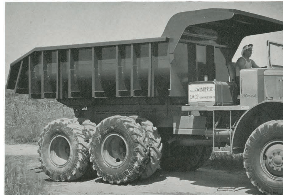
Monster Mack swamp dumpers, now working for Wunderlich-Okes Construction Co. on Panama Canal Third Locks Project, tip the beam at 30 tons when loaded. They're close to 12 feet wide and are powered by 150 h.p. diesel engines. Designed for operation in yielding swamp and muck these big fellows have drive on all six wheels and ride on ten 14.00-24 tires spaced wide apart to secure maximum flotation.
